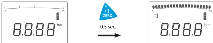
Pushing button #3 for about 3 seconds will produce the instrument's Tare Calibration. The display will show the message "Tare Cal" for some seconds, after which the instrument will have set the current value on the input transducer as the scale zero value. The widest range of the zero calibration is 10% of the device full scale value. Trying to set the zero at an higher value, tare will be set at the highest value possible (10% of the span).
